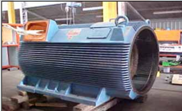
1 MW asynchronous generator
