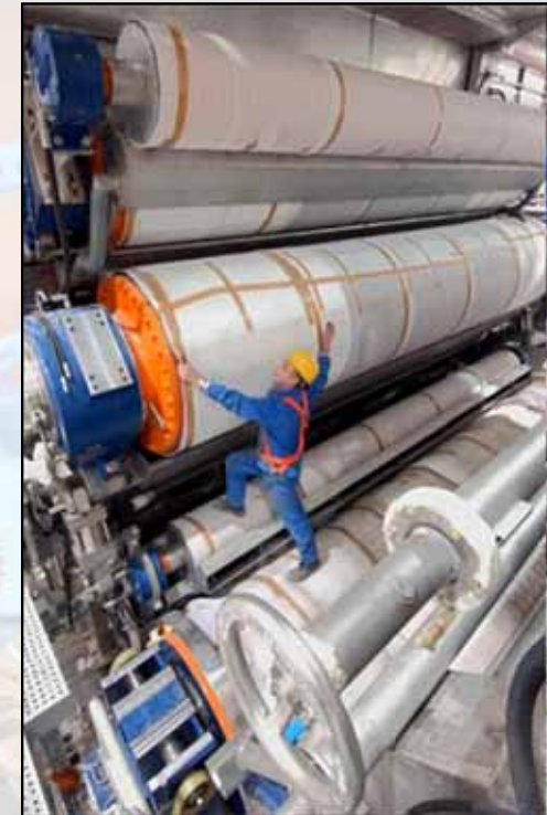
Positioning of absorber cores in a 250kW paper producing machine
