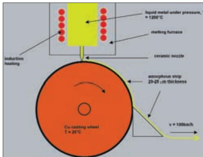
Figure 1: Principle of rapid quenching technology
