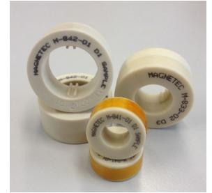
NANOPERM has a curie temperature of about 600°C so it is very temperature stable. The limiting factor for high temperature applications is the plastic fixation material. MAGNETEC offers a new product line of NANOPERM in a high temperature resistant case consists of Dupont Rynite 530L. Rynite 530L have a RTI value of 155°C (UL file E41938) and the temperature class H 180°C (UL file E69939) in combination of selected insulation materials.
