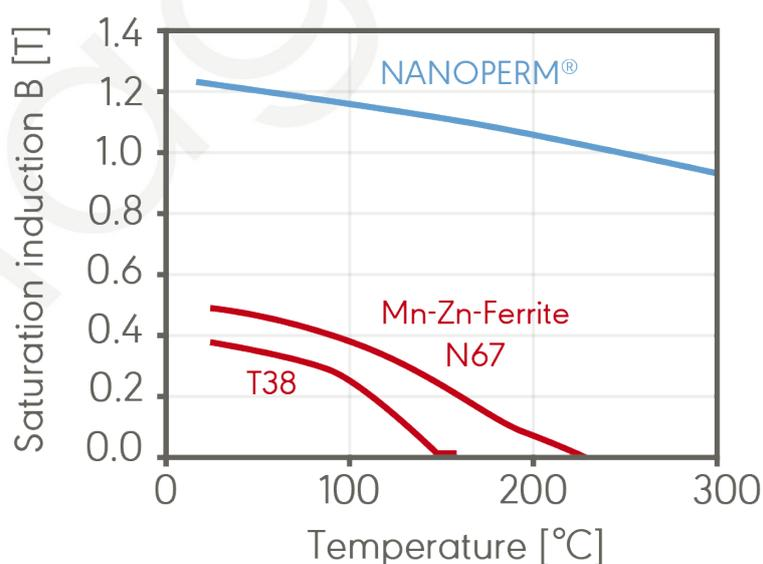
Fig. 4- NANOPERM's high Curie temperature allows for operation at much higher temperatures; that is far superior than other materials.
