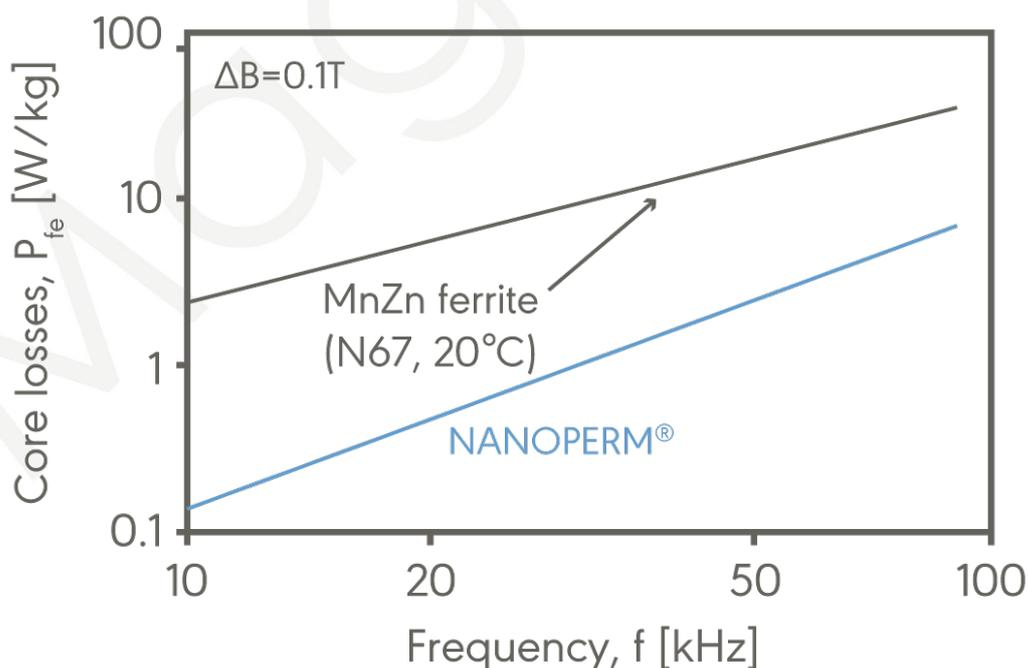
Fig. 2- Core losses of NANOPERM are lower than for common ferrite materials.
