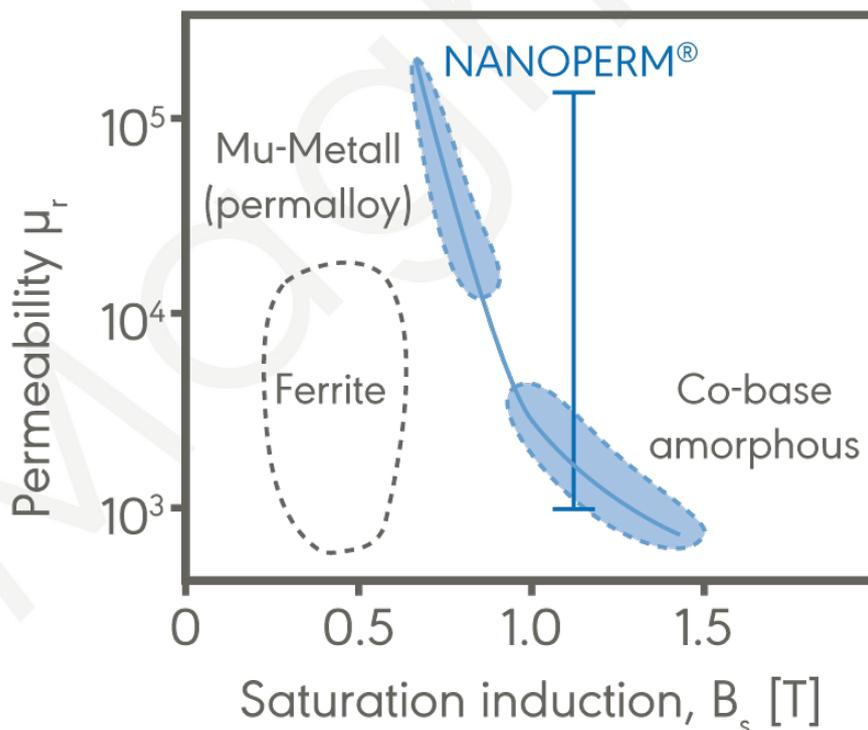
Fig. 1- Typical initial permeability and saturation inductions for low magnetostrictive softmagnetic materials
