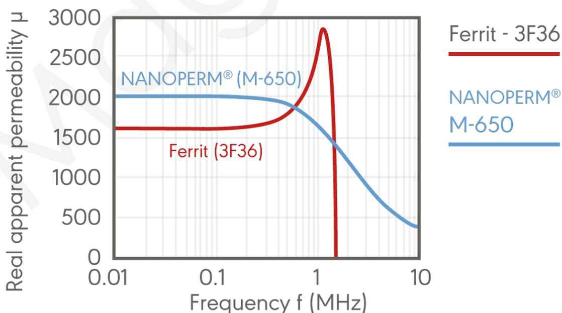
Fig. 3- Permeability vs frequency for a 3F36 ferrite (with toroidal T80 geometry) and a toroidal NANOPERM core (toroidal M-650)
