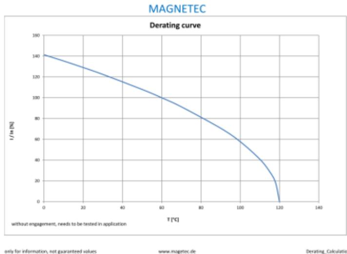
Fig. 1: estimated  $I_{nom\_new}/I_{nom}$  at different ambient temperatures
