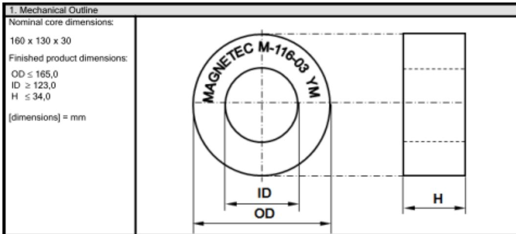
**Nominal core dimensions** are the informative mechanical dimensions (outer diameter x inner diameter x height) of the round magnetic core (in case of a not round shape core, it is the equivalent round core size)
